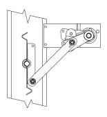
Section of drive device driven to blade closed position by external power source (actuator)
