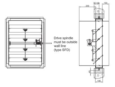
When the damper is installed into the opening and locked in position with the retaining angles, it is recommended that the angles must overlap the opening by at least 25 mm<sup>1</sup> to ensure that the fire integrity of the damper installation is maintained.
